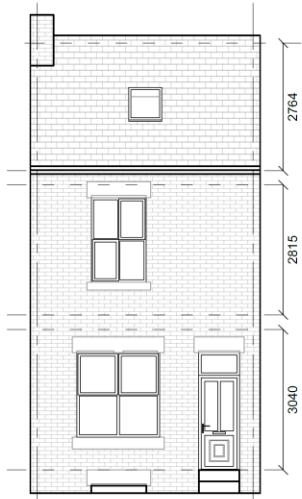
Existing Front Elevation
