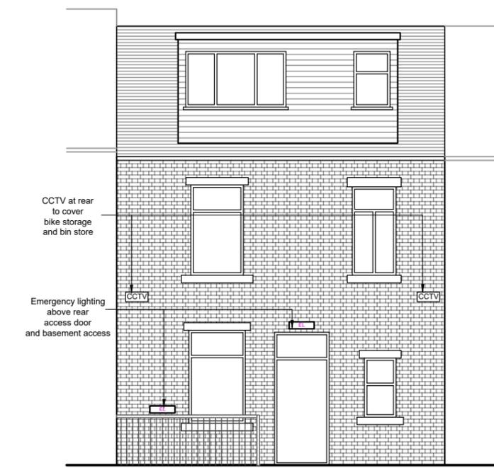
**PROPOSED SECURITY MEASURES ON REAR ELEVATION 1:100 @ A3**
